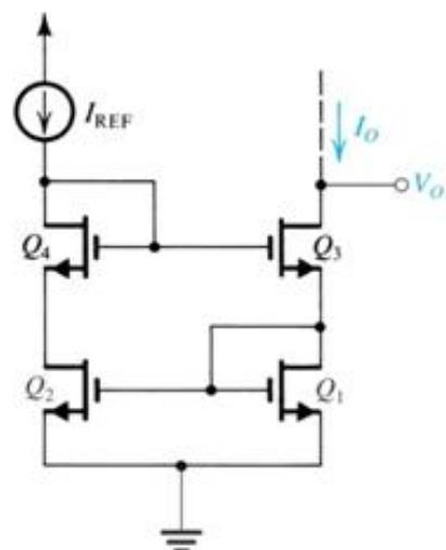
(c) modified circuit to balance the two branches of the mirror and thus avoid the systematic current error resulting from the difference in  $V_{DS}$  between  $Q_1$  and  $Q_2$
