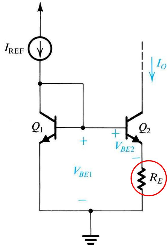
A resistor  $R_E$  is included in the emitter lead of  $Q_2$ . Neglecting base currents, and  $Q_1$  &  $Q_2$  are matched :
