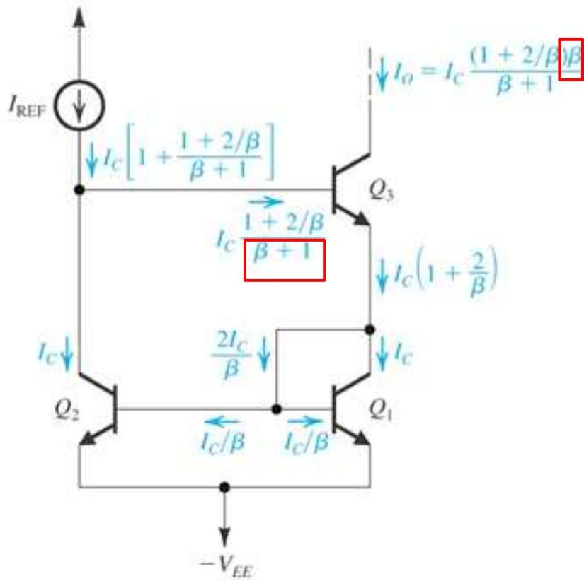
$$I_E = I_B + I_C = (1 + \beta)I_B \quad I_C = \beta I_B$$
