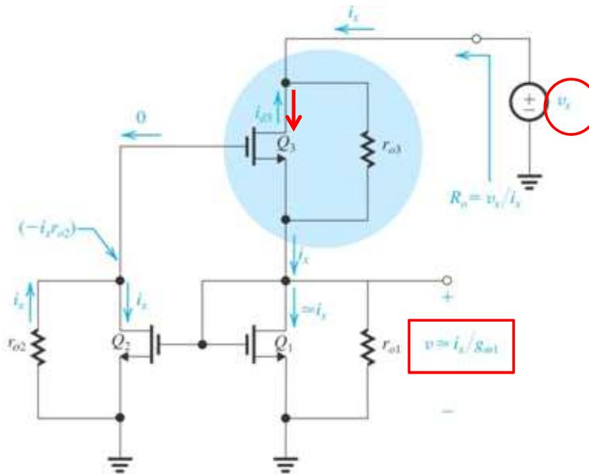
A node eq. at the drain of  $Q_3 \rightarrow$  current through  $r_{o3}$ :
