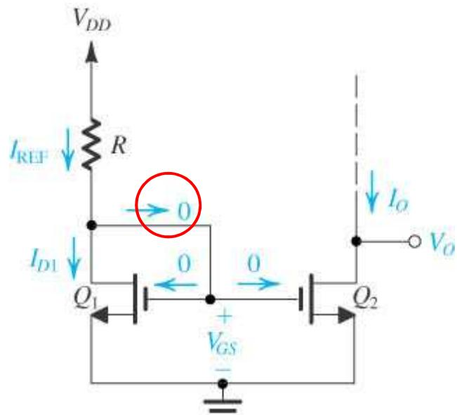
$$I_{D1} = \frac{1}{2} k_n \left( \frac{W}{L} \right)_1 (V_{GS} - V_{tn})^2$$
