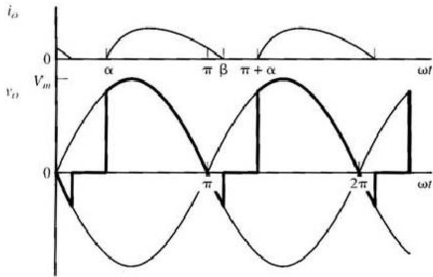
$$i(t) = \begin{cases} \left( \frac{V_m}{Z} \right) \left[ \sin(\omega t - \theta) - \sin(\alpha - \theta) e^{-\frac{(\omega t - \alpha)}{\omega \tau}} \right] & (\alpha \leq \omega t \leq \beta) \\ 0 & \text{나머지 구간} \end{cases}$$
