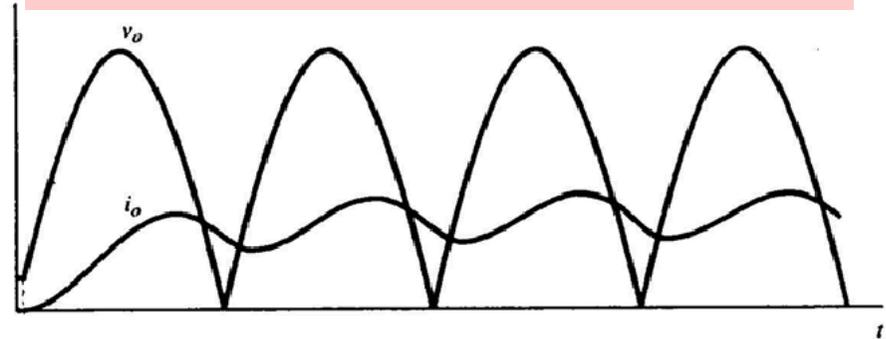
$$v_o(\omega t) = \left( \frac{2V_m}{\pi} - V_{dc} \right) + \sum_{n=2,4,\dots}^{\infty} V_n \cos(n\omega t + \pi)$$
