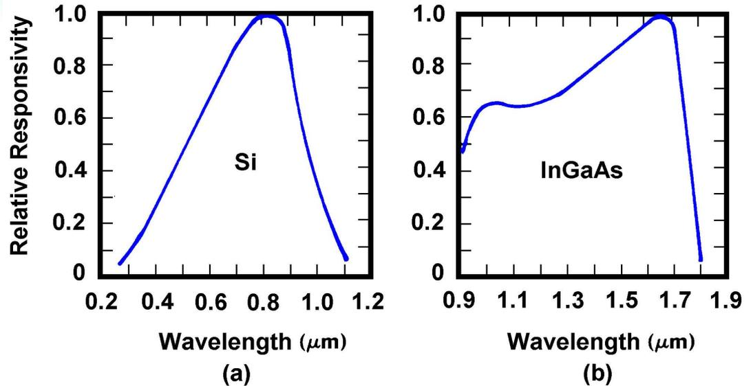
Figure 7-6 Spectral Response Curves
