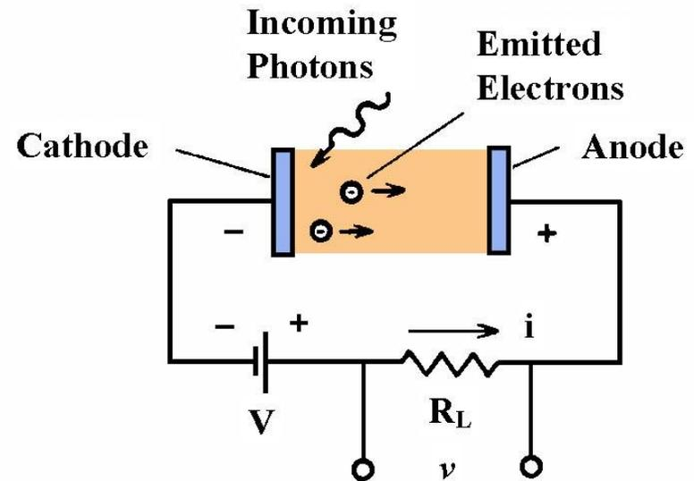
Figure 7-2 Vacuum photodiode
