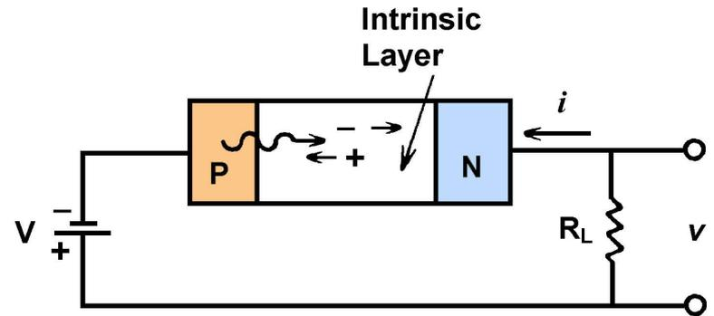
Figure 7-5 PIN Photodiode
