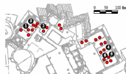
FIGURE 3-7—Experimental Zigbee testbed layout: there are 31 nodes in total, spread over 11 rooms in an indoor office environment. Each unnumbered dot indicates one of 25 Zigbee nodes. The six software-defined radio nodes are shown dark, labeled with numbers.
